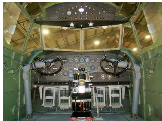
The cockpit fully refurbished with seats still to be installed
